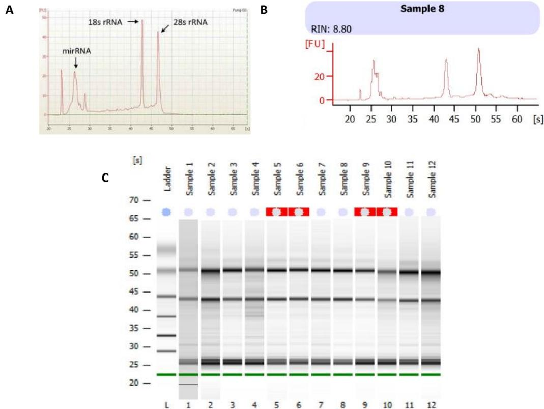
**Figure 31. Total RNA analysis performed on the Agilent 2100 Bioanalyzer.**
